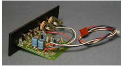
The FRM accessory kit adds 1W FracRak card cage format panel and power connector
